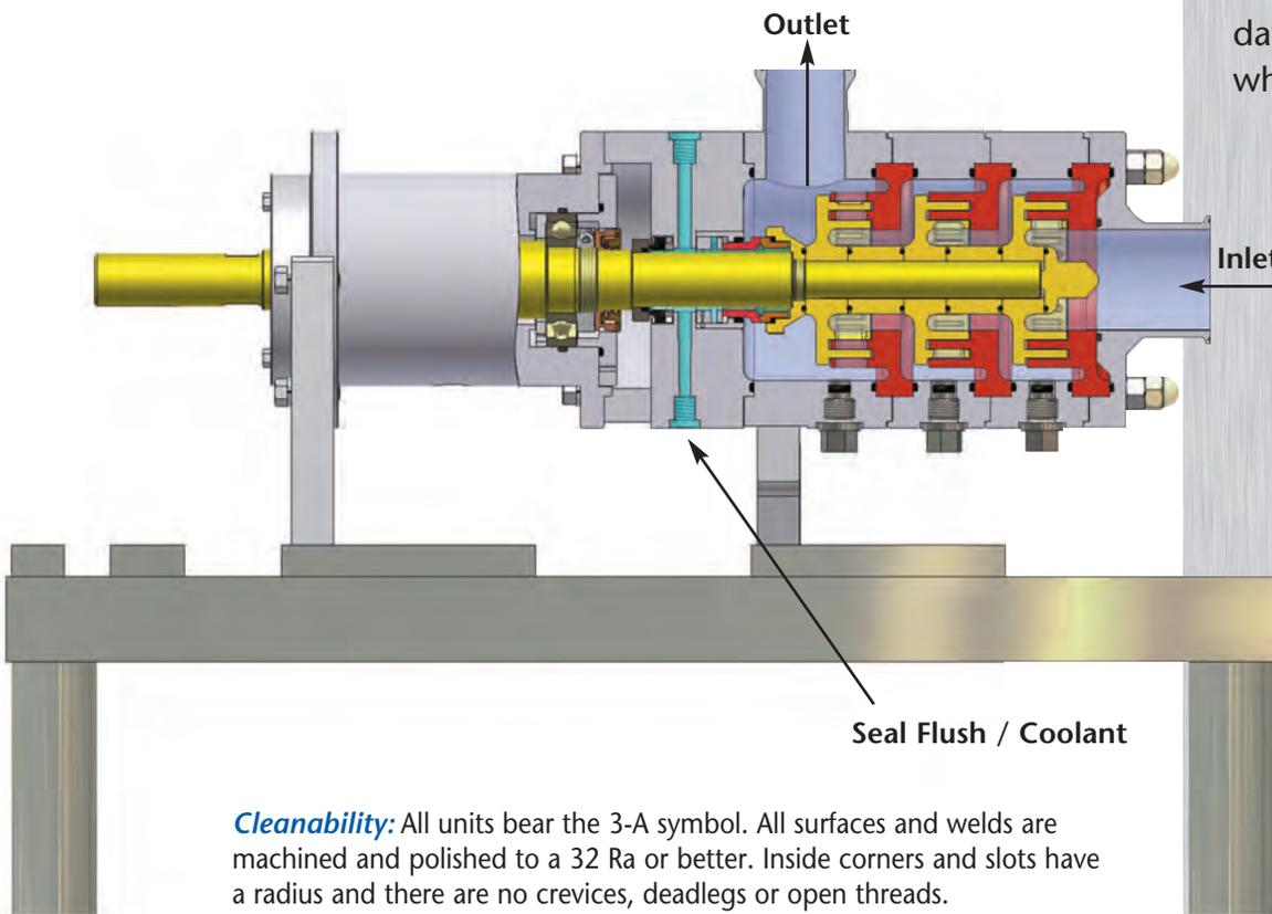
**Cleanability:** All units bear the 3-A symbol. All surfaces and welds are machined and polished to a 32 Ra or better. Inside corners and slots have a radius and there are no crevices, deadlegs or open threads.
